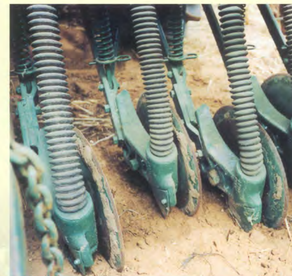
A seed hose adjacent to the disc, delivers seed and/or fertilizer into the bed at a predetermined depth.
